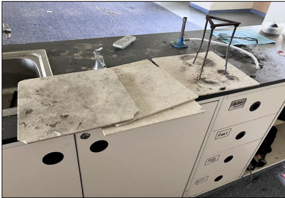
Photograph 3: B00C, CR0003, selected heat insulation pads, fibre cement product, no asbestos detected by analysis.
